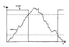
Here's a quick graph to visualize that. The squiggly line represents the voltage at the input, while the solid line shows the voltage at the output. So every time we cross the upper threshold on our way up, and the lower one on our way down, the output changes state. One thing that's very important to keep in mind: no current flows into the sensor! It's really just sensing the voltage without affecting it.
