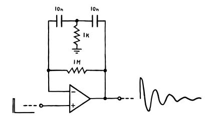
So let's look at how this works. We'll assume that the voltage at the op amp's non-inverting input quickly jumps from 0 to 1 V. Now, to reach a state of balance, the op amp will try to push the voltage at its inverting input up to 1 V as well. For that, it'll increase its output voltage to 1 V. Initially, this will work just fine, since that voltage pushes straight through the two capacitors and reaches the inverting input that way.
