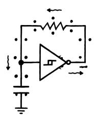
At some point, the voltage above the capacitor will cross the schmitt trigger inverter's upper input threshold, causing it to latch into the high input state. In response, it'll put its output into the low state. Because the capacitor voltage is now much higher than the inverter's output voltage, current will flow out of the cap and back into the output.
