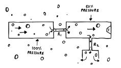
A voltage divider is really just two resistors set up like this: input on the left, output on the right. If R1 and R2 are of the same value, the output voltage will be half of what the input voltage is. How does it work?
