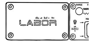
Here, you can insert useful mini-devices that we sell separately. If you don't have any devices to plug in right now, use the included **protection panel** to cover the slot.
