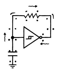
Until we hit the lower input threshold, the inverter latches into the low input state, and the whole process repeats. At the inverter's output, this gives us a square wave whose frequency depends on the size of both resistor and capacitor: increasing either will decrease the frequency, because it takes longer to charge and drain the cap.<sup>3</sup>
