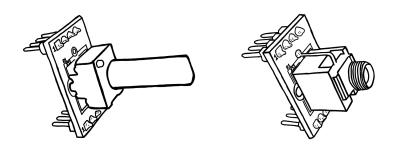
Using the 2x4 pins below the PCBs, you can now plug your interfacing elements into the 2x4 headers at the bottom of the device. You'll notice that there are some helpful notes on the device itself that explain how the individual interfacing elements are connected to the headers above. We'll break this down by looking at an example.
