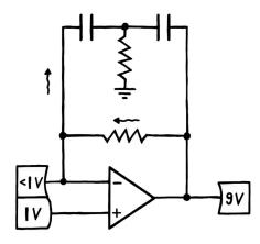
At some point, this process will add more voltage on the left as we lose on the right, causing the whole mechanism to kick into reverse gear. Now, the op amp will start dropping its output voltage to try and course correct. Only problem is that this will pull current out of the first cap, and subsequently up from ground, increasing the voltage between the two caps and also at the inverting input. Which forces the op amp to reduce its output voltage even further.
