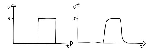
We now know that the resistor acts like a flow-restricting narrow pipe, while the capacitor acts like a charge-storing balloon. So let's say that the input voltage suddenly jumps from 0 V to 5 V. Unlike before, that voltage will now cause current to flow through the resistor and into the capacitor, filling it up.
