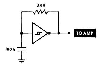
In case you don't know what a schmitt trigger inverter does: you can think of it as two separate things. On the left, there's a sensor that measures voltage. On the right, there is a current pump. The current pump's operation is controlled by the sensor. Whenever the voltage probed by it is below a certain threshold, the current pump will be working. If the voltage is above a second threshold, the pump won't be working.
