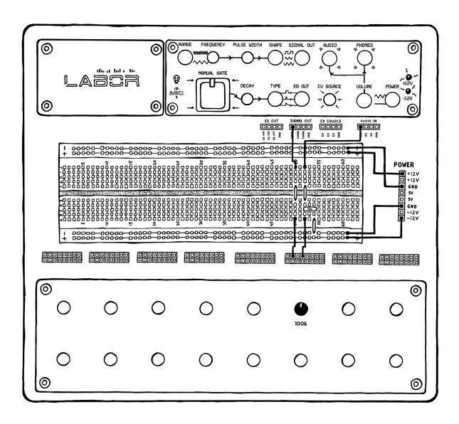
We grab Labor's oscillator from the **SIGNAL OUT** header, route it through the 100k potentiometer plugged into the interfacing section before connecting it back to the breadboard. Here, we then add a 10n capacitor going to ground, before routing the signal to the **AUDIO IN** header.
