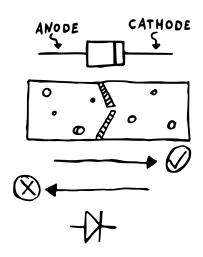
Diodes are basically like one-way valves. Current can only pass through in one direction – from anode to cathode. That direction is indicated by the arrow in the diode symbol and by a black stripe on the diode's casing. So any current trying to move in the opposite direction is blocked from flowing.
