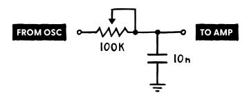
If we arrange them like this, any signal we feed into the input on the left will have its overtones removed to varying degrees, depending on the amount of resistance we dial in. In case you're confused as to how this works: let's dissect this little circuit. First of all, we'll take a look at what a resistor (i.e. our potentiometer) does in this scenario.
