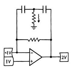
And this would continue until the op amp runs into the upper supply voltage – if it weren't for the bridge resistor between output and inverting input. Because as the op amp pushes harder and harder, that resistor allows a small current to charge up the second cap from the other side.
