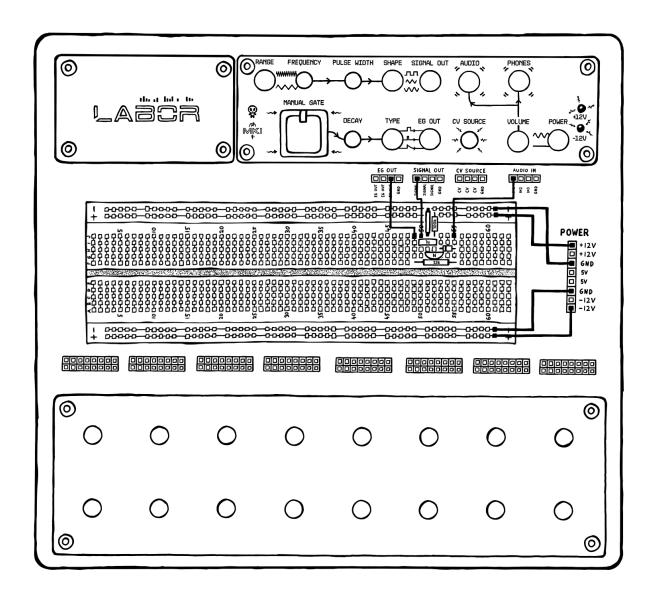
First, we grab Labor's oscillator from the **SIGNAL OUT** header and route it through a 1  $\mu$ F capacitor on the breadboard. On the other side, add the NPN transistor, connect its base to the positive rail using a 100k resistor and its emitter to ground. Next, grab Labor's envelope generator from the **EG OUT** header and connect it to the transistor's collector via a 33k resistor and a 1N4148 small signal diode. Finally, connect the VCA's output to the header labeled **AUDIO IN**.
