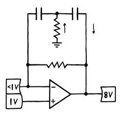
Eventually, we'll again reach a tipping point where the whole mechanism reverses. Only this time, it'll be at a slightly lower output voltage. **That's because with every charging and discharging cycle, we lose a bit of the momentum we initially put in**. The circuit behaves kind of like a pendulum that way.
