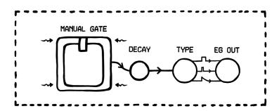
It's controlled by the mechanical push button labeled **MANUAL GATE**. Use the **TYPE** switch to select an output type, then press the button to trigger the generator. The button's LED will light up in sync with the output voltage generated. If you selected the envelope type, you can additionally control its decay via the **DECAY** knob.
