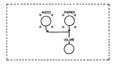
If you connect a signal from the breadboard to the header labeled **AUDIO IN**, you can pick up an amplified version at the jack sockets labeled **AUDIO** and **PHONES**. (The former sends out a line level signal, while the latter is able to drive headphones.) You can control the output volume via the knob labeled **VOLUME**. Finally, next to the utility section, you'll find Labor's **expansion slot**.
