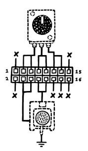
Knowing this, we can work out which pin connects where for our pot & socket – see the illustration on the left. Any pins marked with an **X** are inactive and don't connect anywhere. Note that the jack socket is automatically hooked up to the ground rail – no need to handle this yourself. Using the included jumper cables, you can now connect your interfacing elements to any point on the breadboard.
